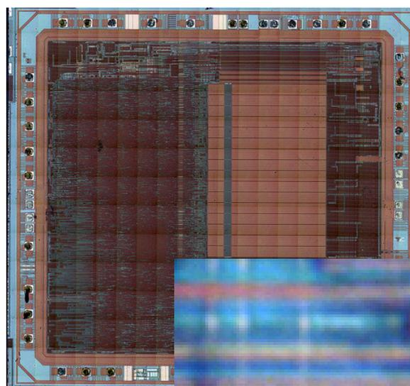
*Figure 1: Image file example of an off-the-shelf device. Actual image is larger than 1GB and contains sufficient details to identify functional blocks of the device and (zoom-on in right bottom corner) even locate nodes of interest for contacting.*
