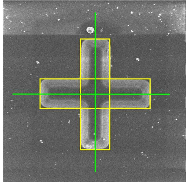
Figure 2: Box pattern overlay, aligned symmetrically with the reference object. Interception point of two boxes with zero width indicates location of the center of the reference, allowing repeatable lock even on damaged reference objects.
